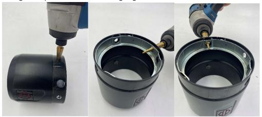
c. Fit the tips to the new mufflers to check mounting holes. You should not be able to see any tip material in the mounting hole. If you do, adjust the holes so that you don't.
