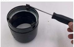
d. Remove the inner mounting ring from the tip. This is a very tight fit, so you may need to use a hammer and punch to remove it.
