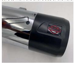
c. With the holes marked, insert the inner mounting ring onto the tip. Be sure to align one of the previous holes with one of the new marks on your tip. The flat side of the mounting ring should be facing the exit of the muffler.
